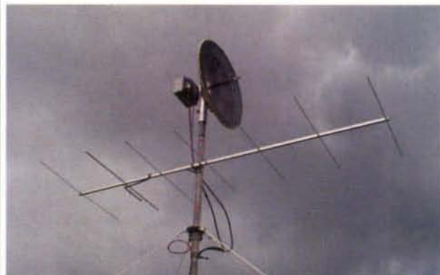
Fig. 1: The 10GHz dish and 144MHz antenna at the station of G4ZXO/P.
