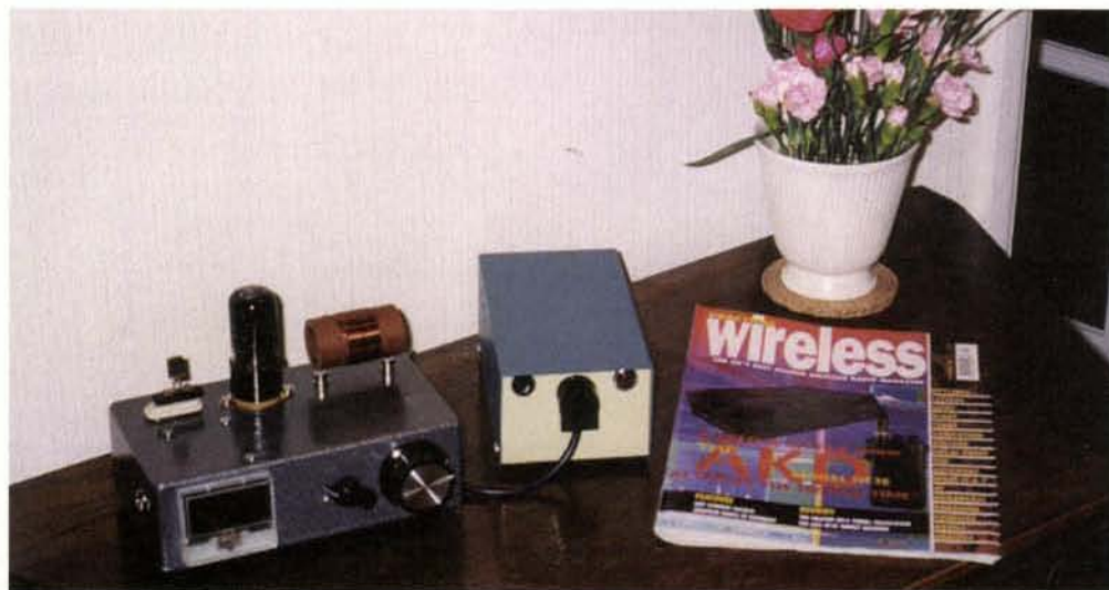
Fig. 3: Photograph showing the (very neat-looking) 6V6GT one-valved transmitter, from an article incorporating a classic design and published in the December 1997 PW (see text).
