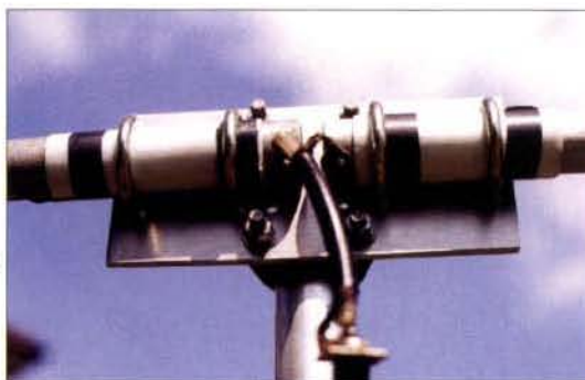
Fig. 6: Driven element centre insulator section. The elements are insulated from the plate and the U-bolts with thick PVC insulation, which is taped to the elements before fixing in place.
