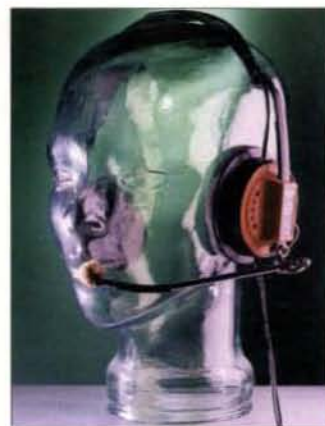
Fig. 5: A home-made boom microphone is easier to make than you think. See text for more details.
